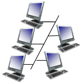
Shared wire (e.g., cabled Ethernet)
