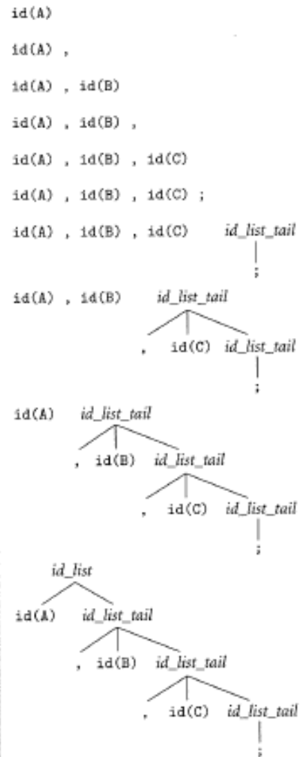
Figure 2.13 Top-down (left) and bottom-up parsing (right) of the input string A, B, C; . Grammar appears at lower left.
