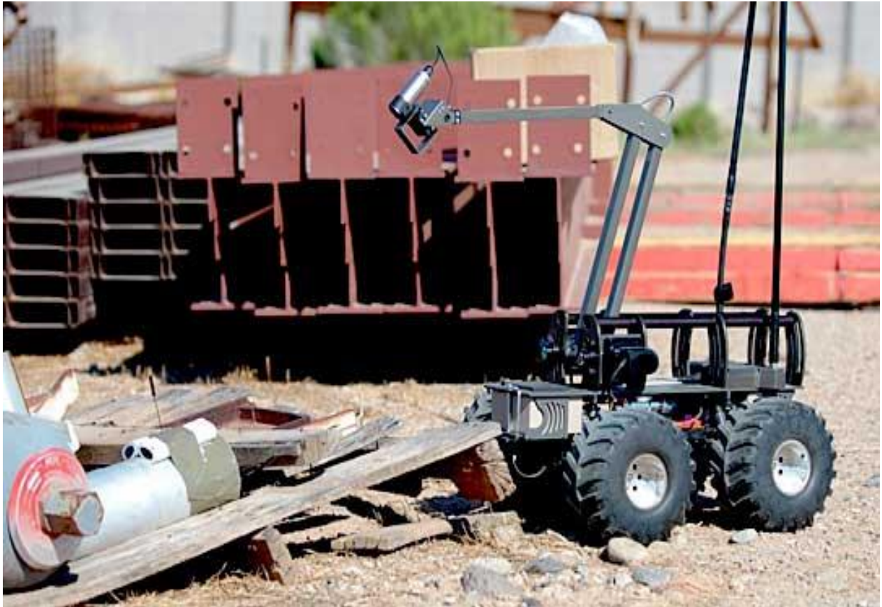
(Figure 3) MARCbot investigating a possible mine without toughing the threat area.
