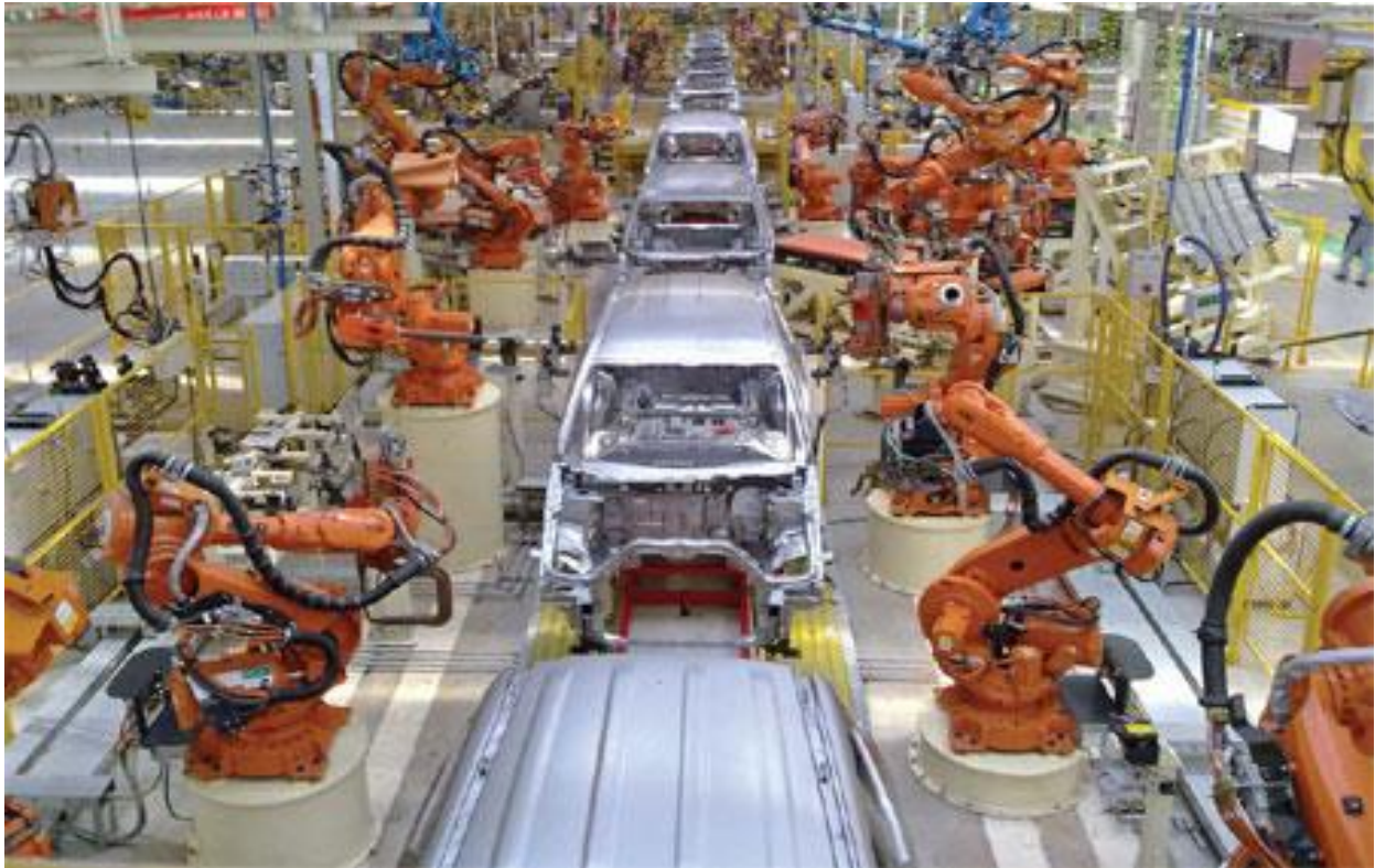
(Figure 1) Car production robots that takes turn in finishing the task then move one the driving belt to the next job.
