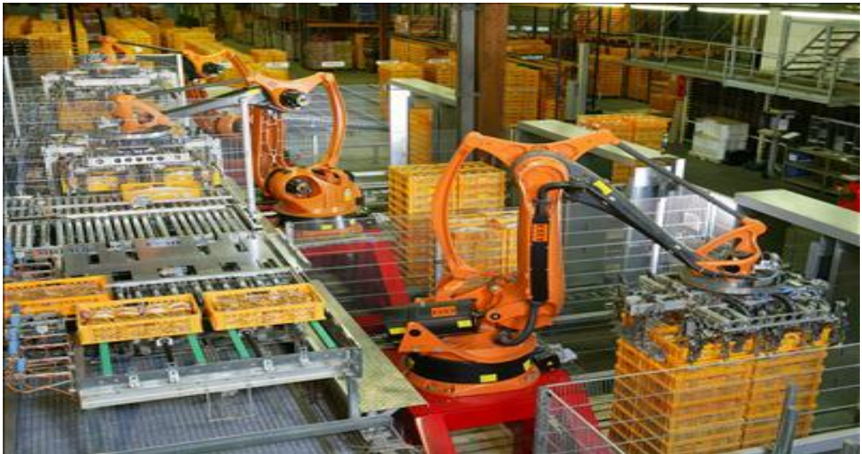
(Figure 2) Palletizing robots pick up the finished food package.
