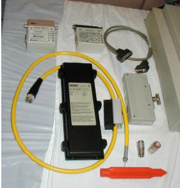
Thick Ethernet cable (yellow), 10BASE-5 transceivers, cable tapping tool (orange), 500m maximum length.
