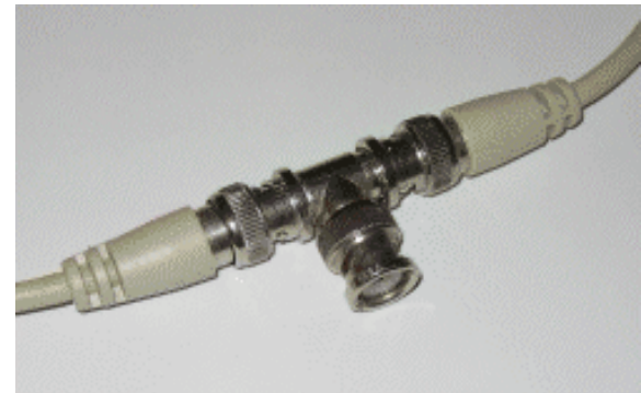
Thin Ethernet cable (10BASE2) with BNC T-connector, 185m maximum length.
