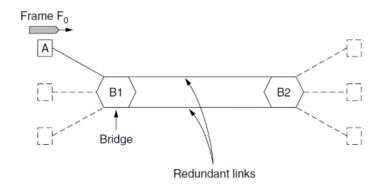
Packets would get stuck in a loop going between B1 and B2 (at least until the packets die or B1/B2 learn where D actually is).
