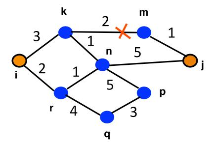
a) Suppose the link between nodes k and m fails. Before the failure, what is the shortest path from node i to node j? What is the new path after the failure (after the routing protocol converges)?
