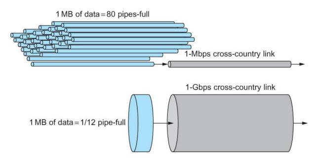
1 MB file, 1-Mbps link with RTT of 100ms, 80 full pipes 1 MB file, 1-Gbps link with RTT of 100ms, 1/12 of a full pipe
