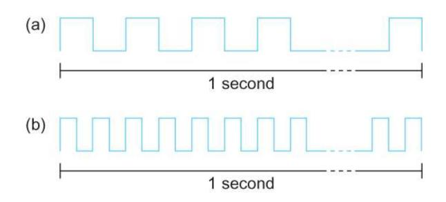
(a) bits transmitted at 1 Mbps (each bit is 1 x 10<sup>-6</sup> seconds wide)
